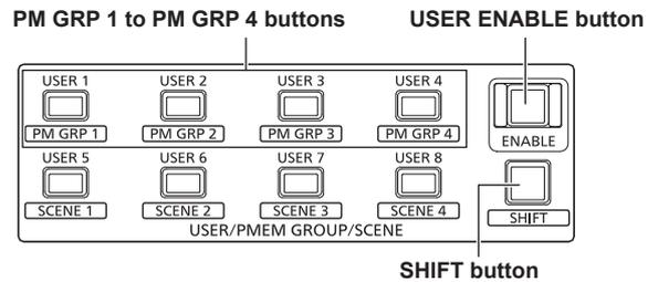
1. Press the SHIFT button to turn on its indicator.
