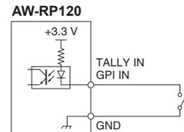
For the cameras registered to the "1. CAM OUT1" to "10. CAM OUT10" items in GPI OUT menu [45], the selection states on the unit can be output to GPI OUT1 to GPI OUT4.
