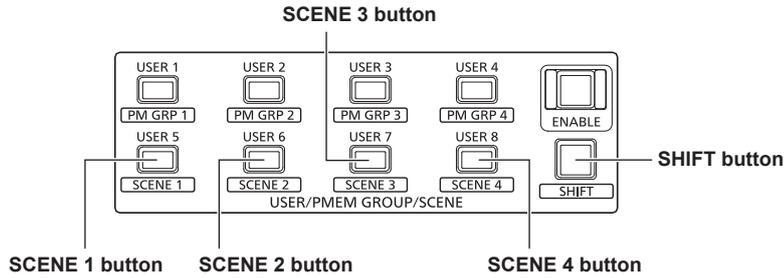
1. Press the **SHIFT** button to turn on its indicator.
